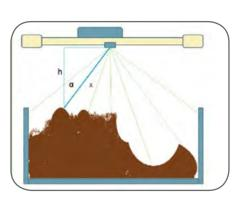
Each time that the waste handling crane cover predefined positions, either forward and backwards, it carries out a scanning and refresh heights data on each position. 垃圾吊每次经过预设位置时, 无论是向前还是向后, 扫描装置启 动,并更新每个位置的高度数据。
