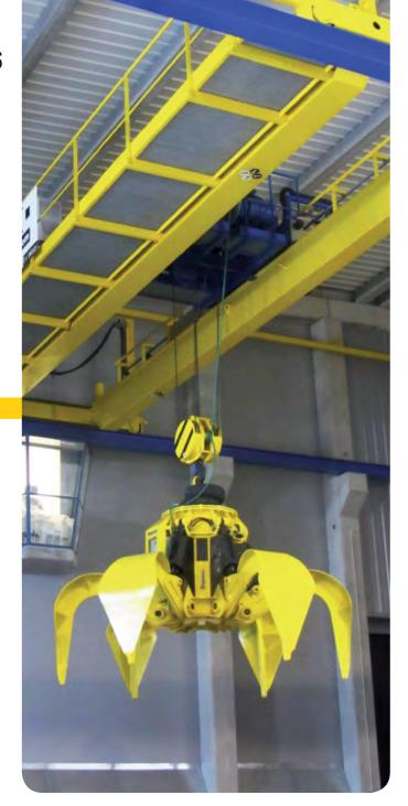
This is why it is necessary to have a special lifting system available with two drums. Both drums must make movements, completely determined by a differential combiner, sometimes in the same direction and sometimes in the opposite direction.:
